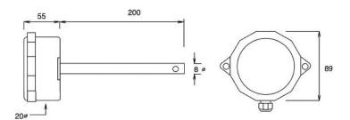
Ensure that the air flows directly through the holes in the side of the probe. The air can enter the holes from either side. Mount away from bends, elbows and turbulent areas. Avoid installi.ng in areas where the temperature in the duct changes rapidly.
